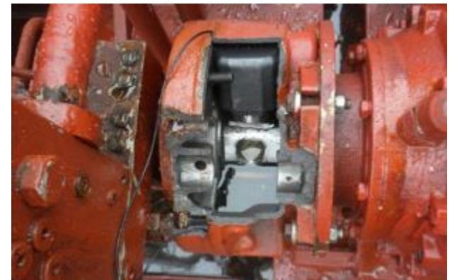
Hydraulic motor with broken cover plate
