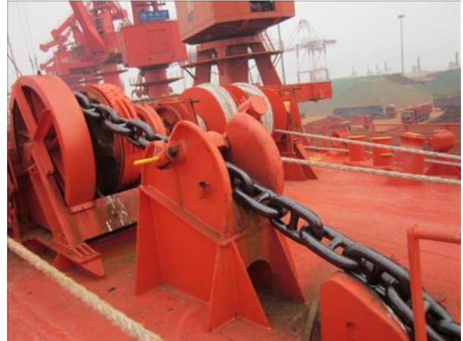
Windlass and chain stopper with guillotine bar
