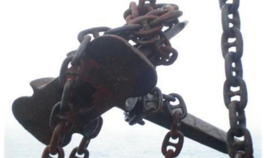
Anchor with fouled chain
