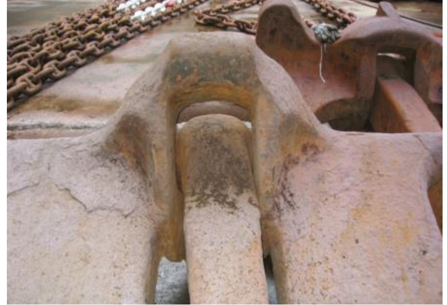
Two anchors of the same ship are of different types , hence one is a second hand anchor
