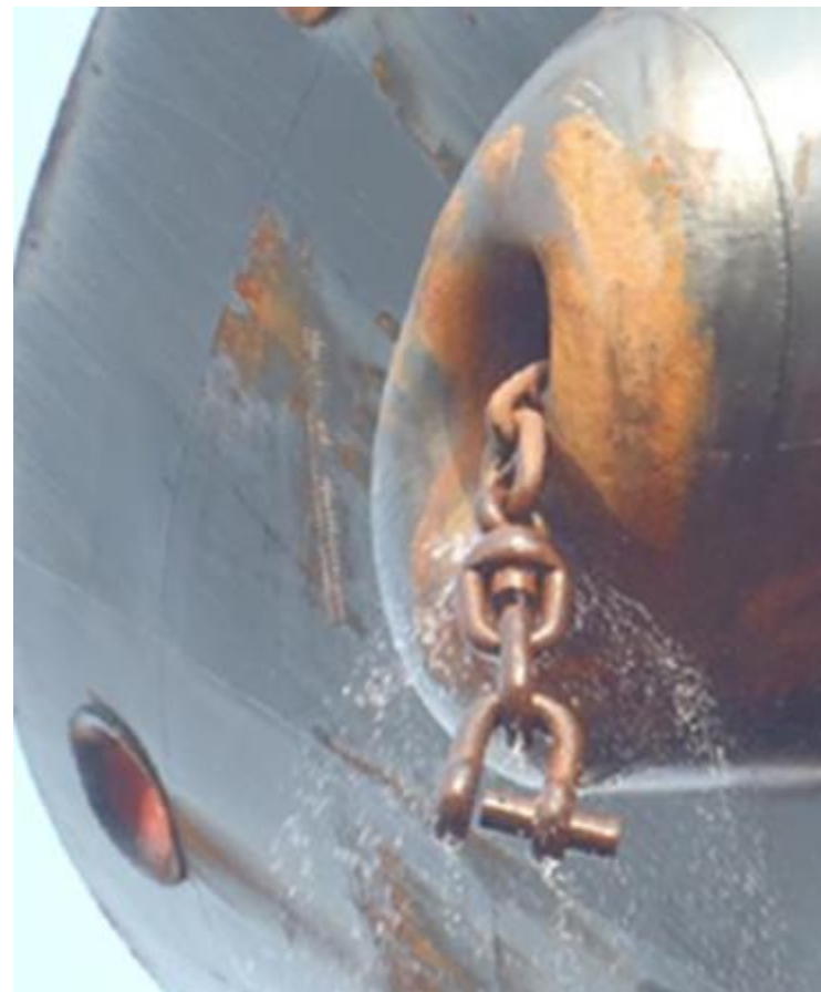
Anchor lost due to D-link opening up
