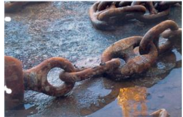
Heavily worn and bent anchor chain links
