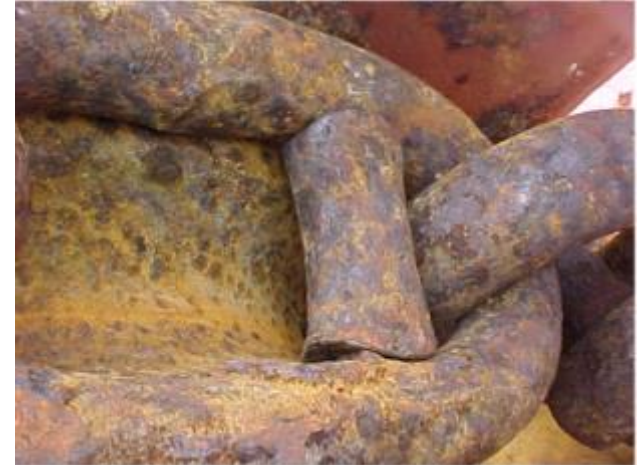
Loose and dis-located studs
