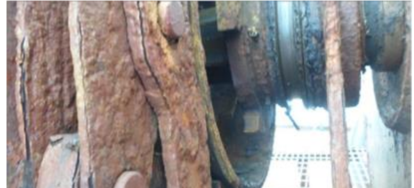
Windlass in poor condition
