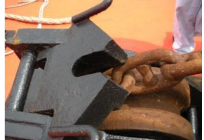
The pawl does not fit the chain
