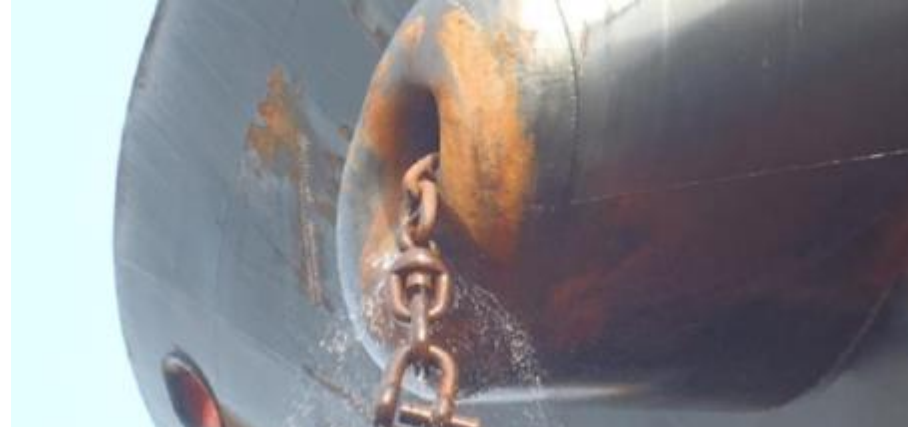
Anchor lost and D-Link securing bolt loose
