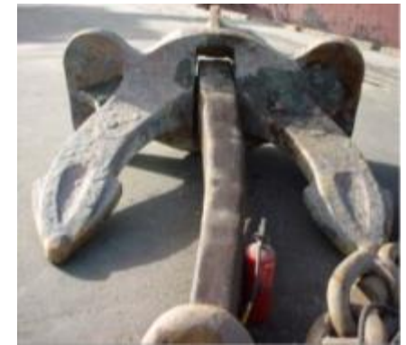
Bent anchor shank may be straightened
