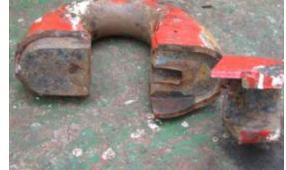
Broken Kenter shackle
