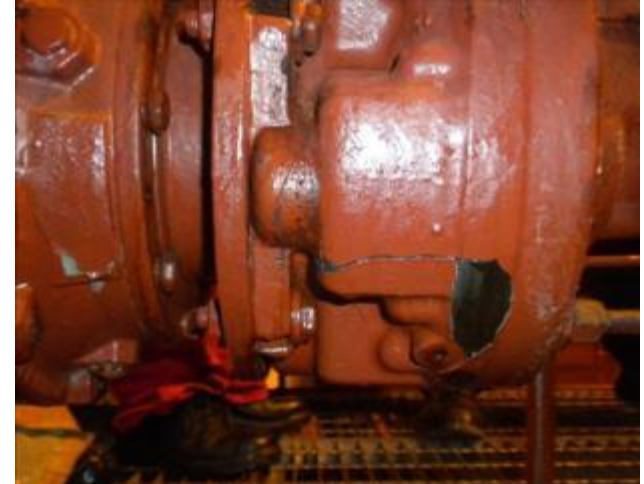
Hydraulic motor exploded during heaving anchor in heavy weather
