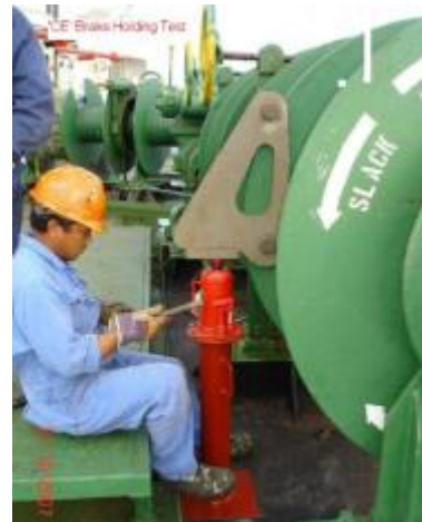
Brake band jack up test
