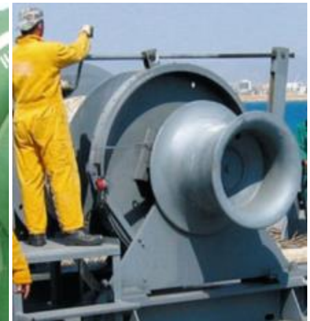
Applying the brakes while lowering the anchor
