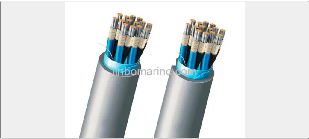
S14 BU(c) Halogen-free Fire-resistant Offshore Instrumentation & Communication Unarmoured Cable with collective screen
