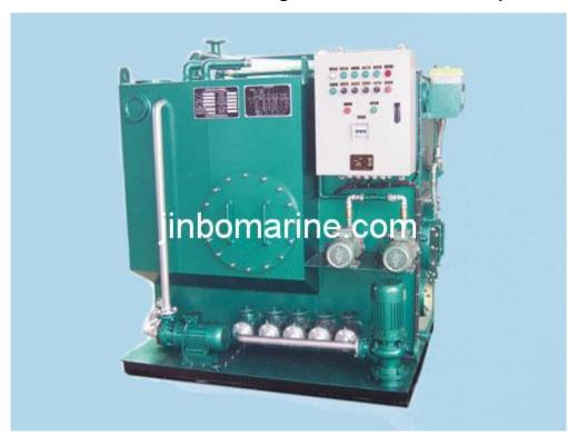
The plant is applicable to treat the sewage from the onboard ship toilets to meet international standards of discharge.
