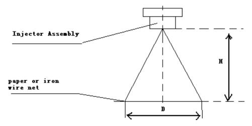
Repeat to pump fuel until you can see clearly a fuel circle or an empty circle in the iron-wire net. Measure height of "H" from the mouth to the net (paper) and diameter of outer circle. Injecting angle may be calculated according to the following formula:
